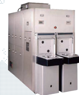
Dry Resist Strip System Lambda300
